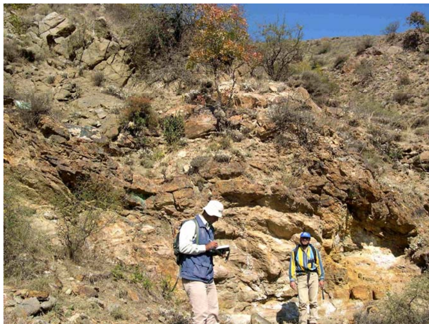
Photo 48. 2m wide malachite and neotocite-stained grey silica vein containing 3% pyrite disseminations (most changed to limonite). Vein trend is 280° with 40° N dip. The granodiorite wallrock is altered to quartz-clay±sericite-limonite for up to 2m from the vein. (Rock Sample No. 84.SAM.90).
