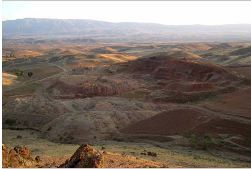
Photo 15. Southwest view of the abandoned Fe-clay mine showing argillic-hematitic alteration of the andesites at the western flank (right upper side) and kaolinite-rich fault zone at the creek.
