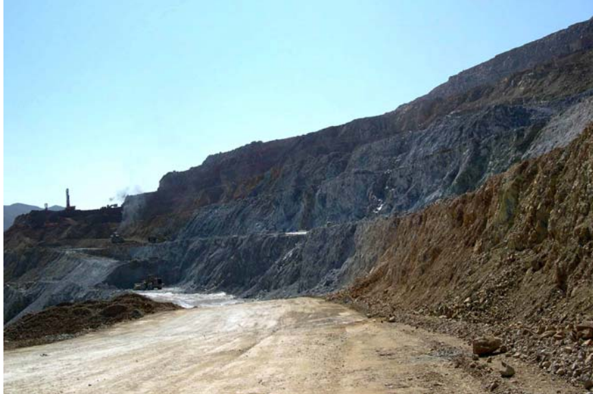
Photo 22. Unoxidized (grey in color) argillic-1% pyrite altered biotite feldspar±quartz porphyry (DK1A) dyke cutting oxidized (red brown in color) mineralized quartz monzonite (SP) at 2200-2187.5m ramp.
