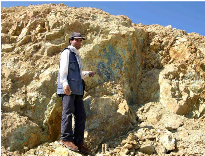
Photo 24. Supergene Cu oxide ore - azurite and malachite along fractures of oxidized phyllic altered quartz monzonite (SP) at 2200-2187.5m ramp.
