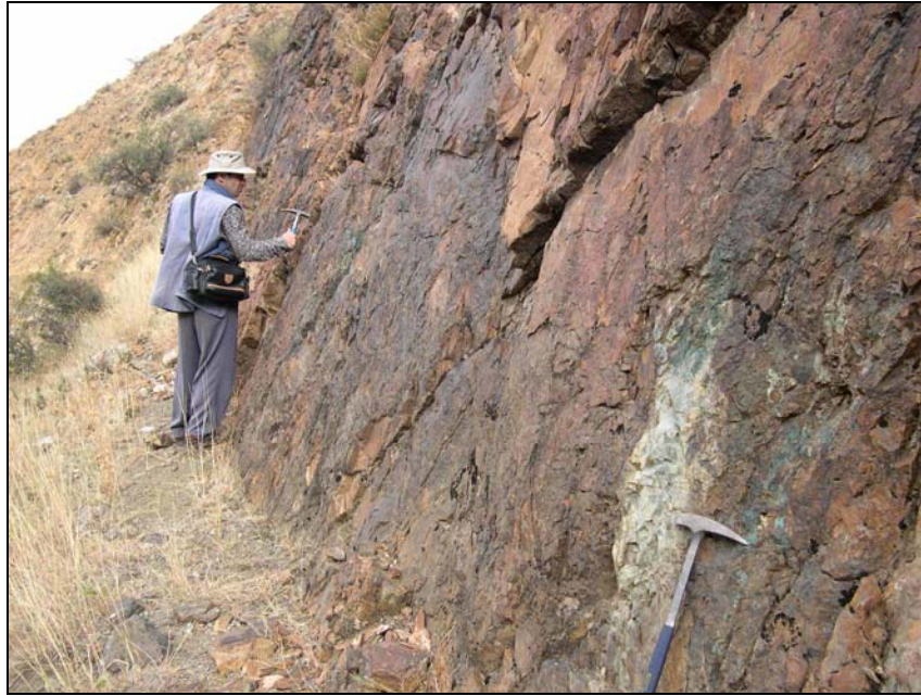
Photo 4. Silicified fault zone, 2m wide, containing 1% pyrite, trace chalcopyrite and malachite stains. Fault gouge (white) indicate post-mineral movement.
