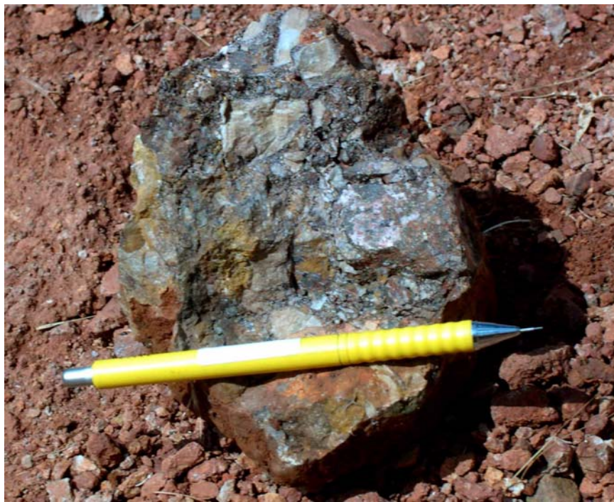
Photo 11. Float of hydrothermal vein breccia with limonite (after sulphide) matrix – possible source of malachite stains.
