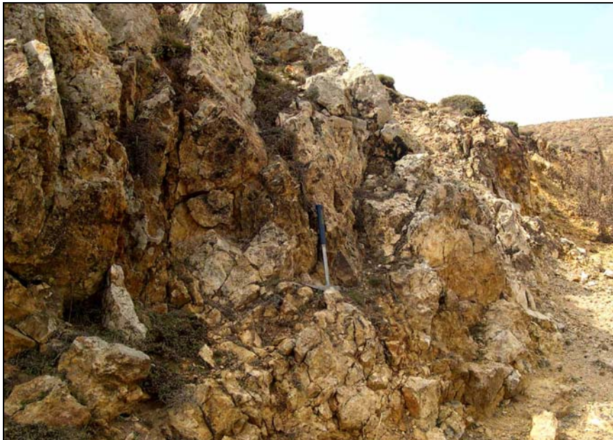
Photo 35. 320° trending epithermal quartz vein zone (white in color), 1m wide, in sericite-limonite altered hornblende biotite diorite. Hydraulically brecciated patches are noted.
