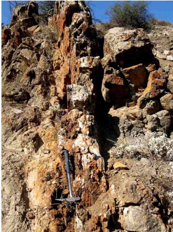
Photo 49. 40cm wide milky quartz vein carrying chalcopyrite and pyrite (almost completely changed to limonite) and minor molybdenite in biotite quartz diorite ((Rock Sample No. 84.SAM.91). Vein trend is N-S with 85° W dip.
