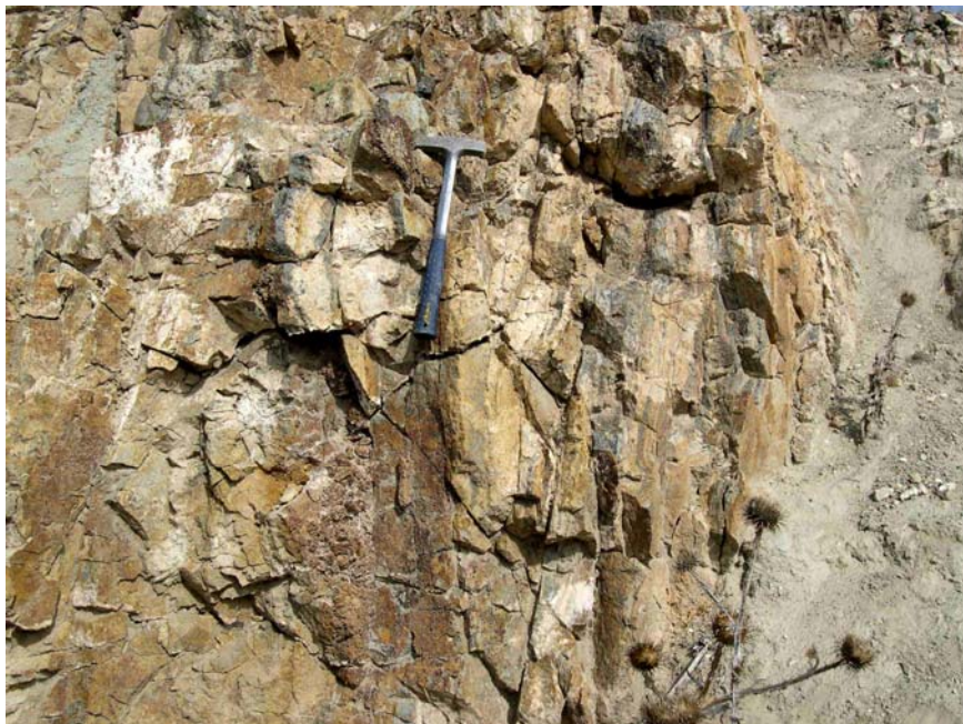
Photo 20. Close up of quartz-limonite (after pyrite) vein (left side – Rock Sample No. 84.SAM.86) and tourmaline vein (right side – Rock Sample No. 84.SAM.87) in sericitized hornblende biotite diorite of Oligocene age.
