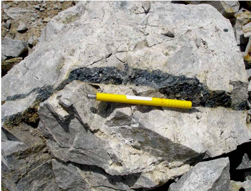
Photo 23. Supergene Cu sulphide ore - phyllic altered quartz monzonite (SP) with 2cm wide chalcocite veinlet and pyrite fracture fills cutting 3-10mm wide milky quartz veinlets at 2200m mine bench.
