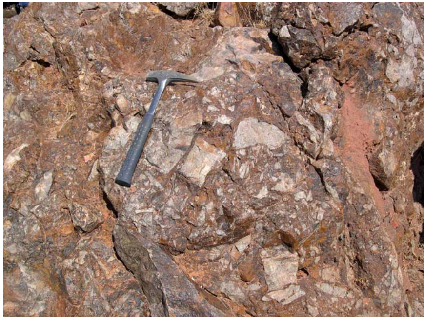
Photo 14. Close up of the chalcedonic silica hydrothermal breccia containing angular chalcedony clasts in hematitic matrix (Rock Sample No. 84.SAM.58).
