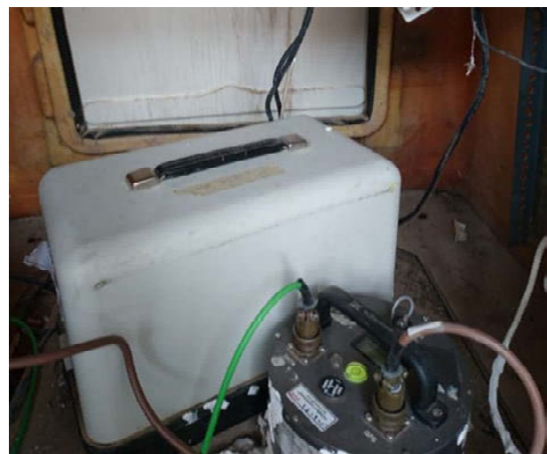
Figure 2. Sarpol-e Zahab station (SSA-2 permanent instrument along with the temporary CMG-5TD instrument).
